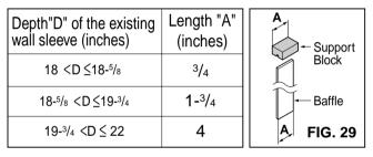
6 Remove the backing from the support blocks and attach them to the inside of the wall sleeve as shown FIG 30. Slide the baffle into slots of the support blocks.
